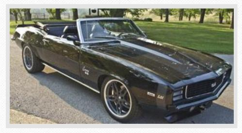
By packing this client's '69 Camaro convertible with an all-aluminum 5.7L LS1 small-block, an overdrive transmission, a four-link rear suspension and disc brakes, Precision Restorations transformed an ordinary musclecar into a modern Pro Touring machine. Thanks to modern technology, it can knock down 20 miles per gallon on the street and clip apexes on a road course.
